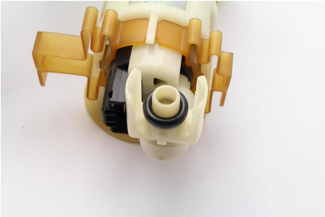
5 – pry the retainer clip from the fuel sock and separate the fuel pump from the pump cage
