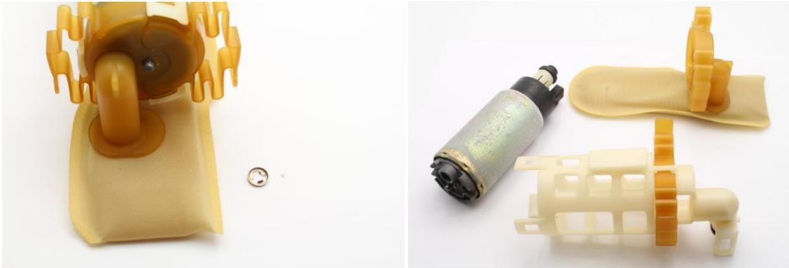
6 – transfer the oring spacer from the outlet of the OE pump to the outlet of the DW65c and install into the pump cage. BOTH ORINGS FROM THE DW INSTALL KIT WILL BE USED ON THE OUTLET OF THE DW65c
