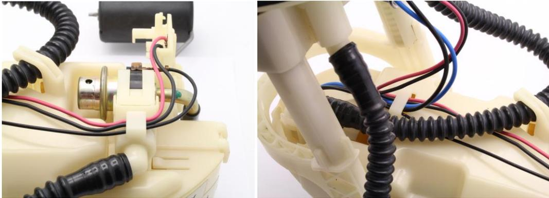
1 – remove wires from their holders and separate the top hat from the assembly
