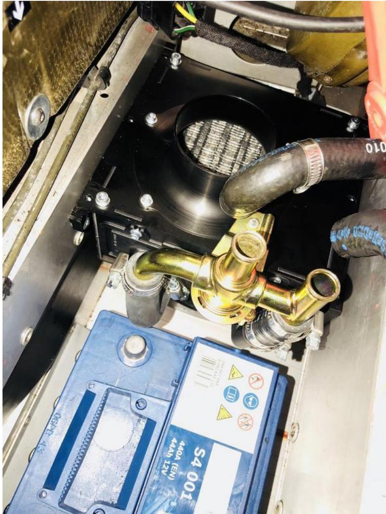
22. Use 6x M4 Cap Head bolts and washers and secure the heater to the brackets – most of these are easy to get to apart from the holes furthest away under the servo, don't worry if you cannot get to a couple of them, the heater isn't going anywhere with 4 or 5 bolts in place.
